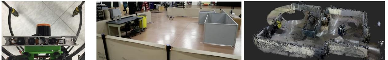
This has further developed into autonomous aerial patrol [33]. Assuming that the probabilistic map diffuses over time, minimizing map uncertainties causes the vehicles to revisit particular areas that were mapped a while ago. The following figures illustrate collaborative 3D patrol for a large building.
