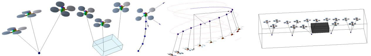
The proposed control systems have been verified indoor flight experiments for stabilization of a point mass [24], stabilization of a rod with two quadrotors [26], and tracking a point mass with a single quadrotor [28]
