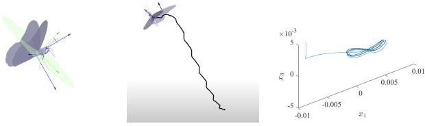
We have proposed supervised learning control, where a neural network learns optimal control trajectories that minimize the tracking error. Due to their ability of consistent generalization, the learned neural network successfully stabilize the complicated flapping motion. More importantly, the training process is carefully
