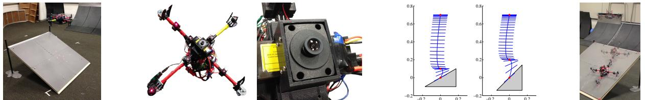
Another interesting experiment is rejecting the wind disturbance caused by an industrial fan [10, 11], where the unknown effects of turbulent wind is compensated by neural networks. First, the advantages over conventional adaptive control were demonstrated (left), followed by performing an aggressive maneuver under the wind gusts (right).
