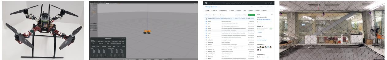
**Indoor Flight Experiments** For indoor flight experiments, the position of the quadrotor is measured by an infrared motion capture system. Notable experiments include backflipping [4], and landing on an inclined surface [15, 16], as shown below: the inclination and height of the surface are estimated by capturing a pattern projected by laser points, and the landing trajectory is planned based on the estimation results, before the landing maneuver is executed.
